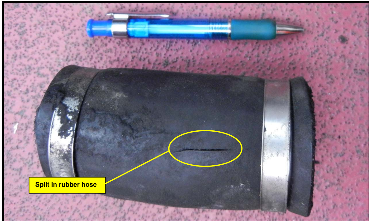
Photograph 1: Split in connecting hose
