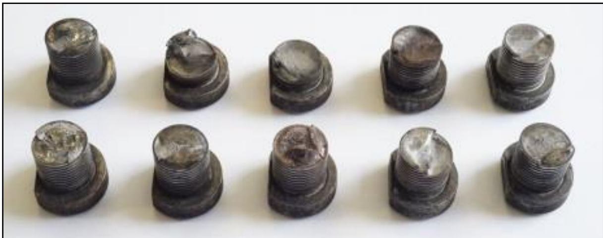
Photograph 4: The broken wheel bolts
