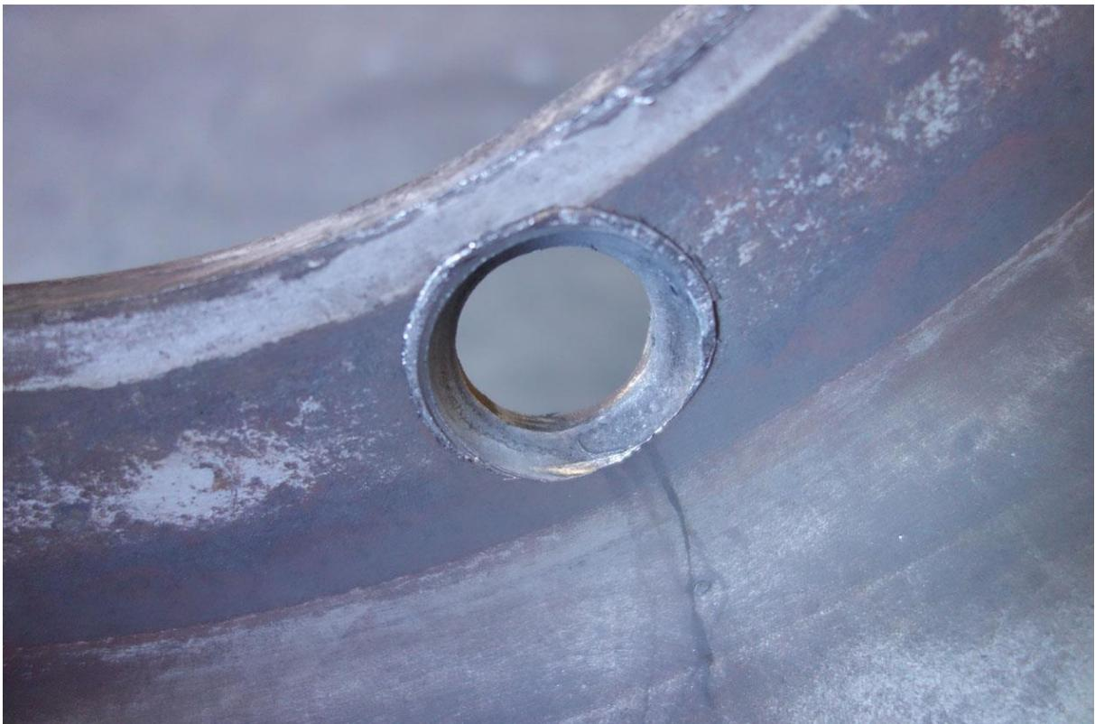
**Photograph 2: Damage around stud hole in wheel**
