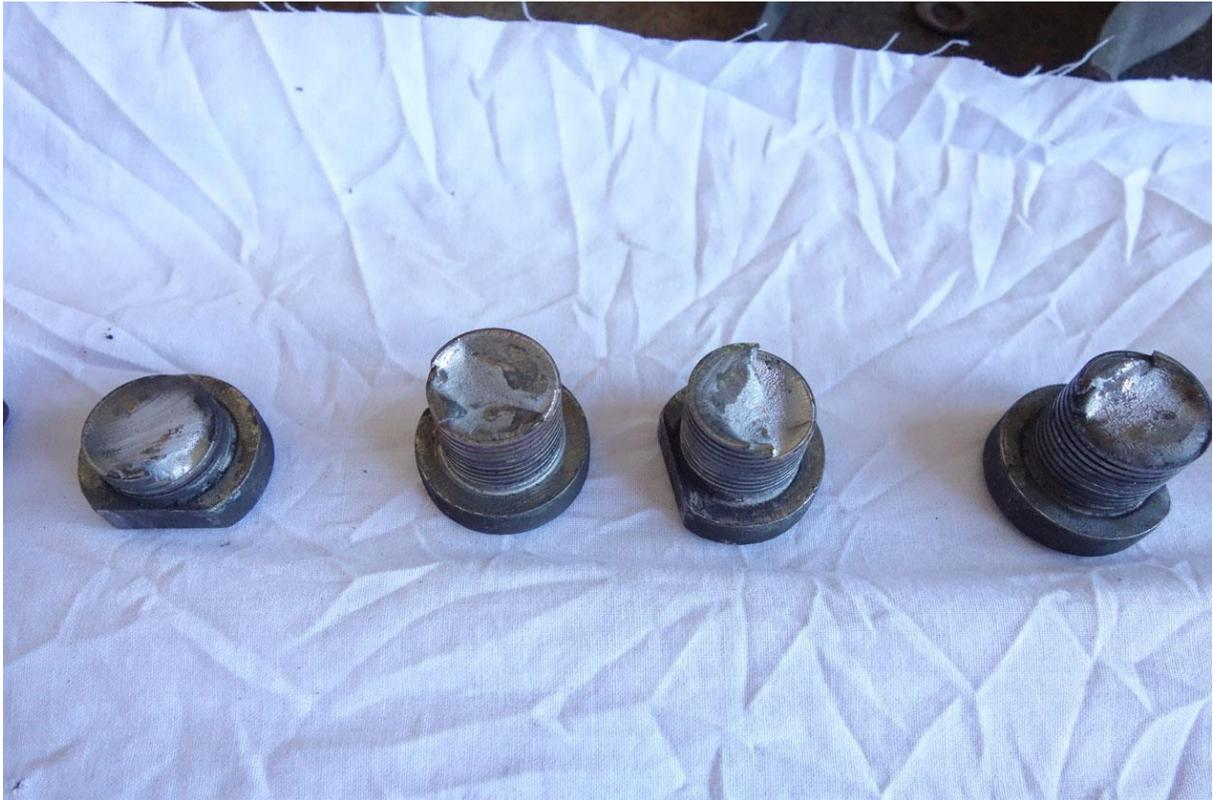
**Photograph 2: Broken wheel studs**
