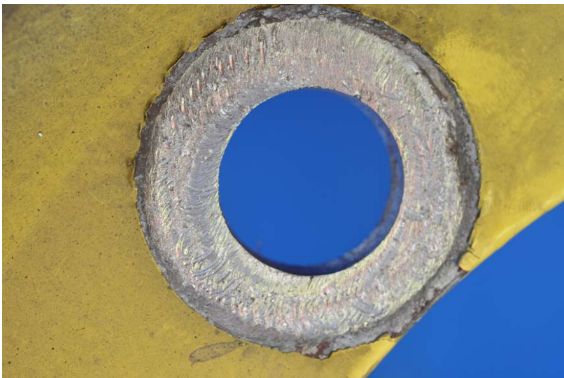
Photograph 7: Close View of Fretting Caused by Loose Nuts
