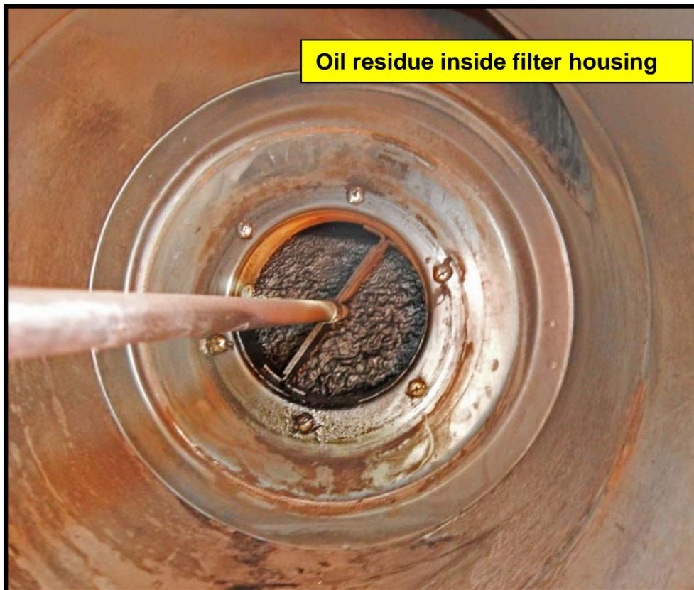
Photograph 3: Inside air filter housing
