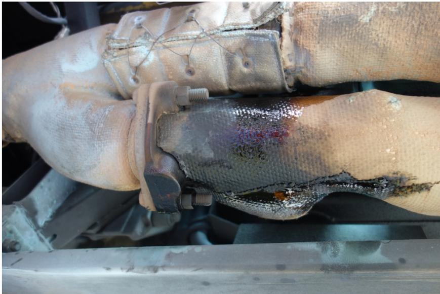
**Photograph 1: Fluid leak onto manifold lagging**
