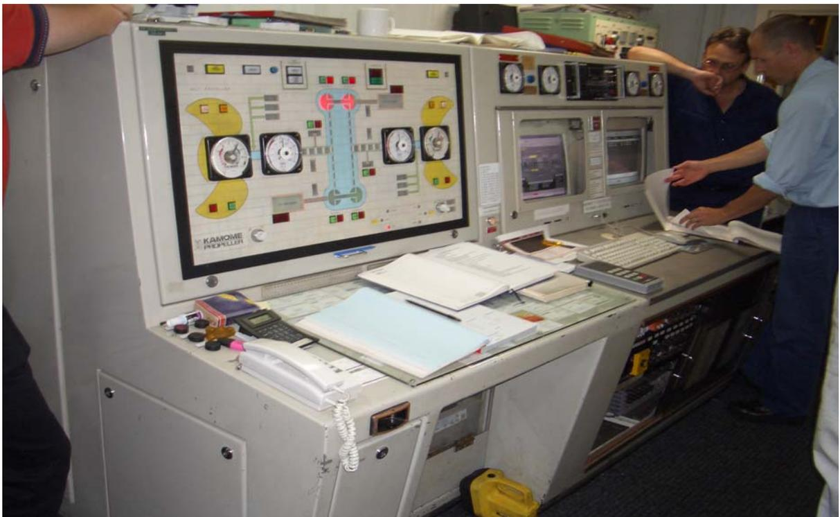
Figure 6 Collaroy's Machinery Control Room (MCR) Mimic Panel and Data Logger Console
