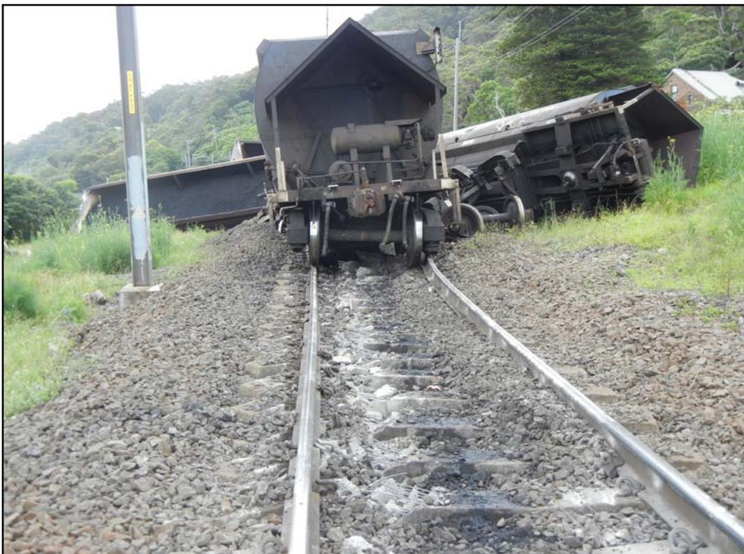
**Figure 1: Derailed wagons and track damage**
