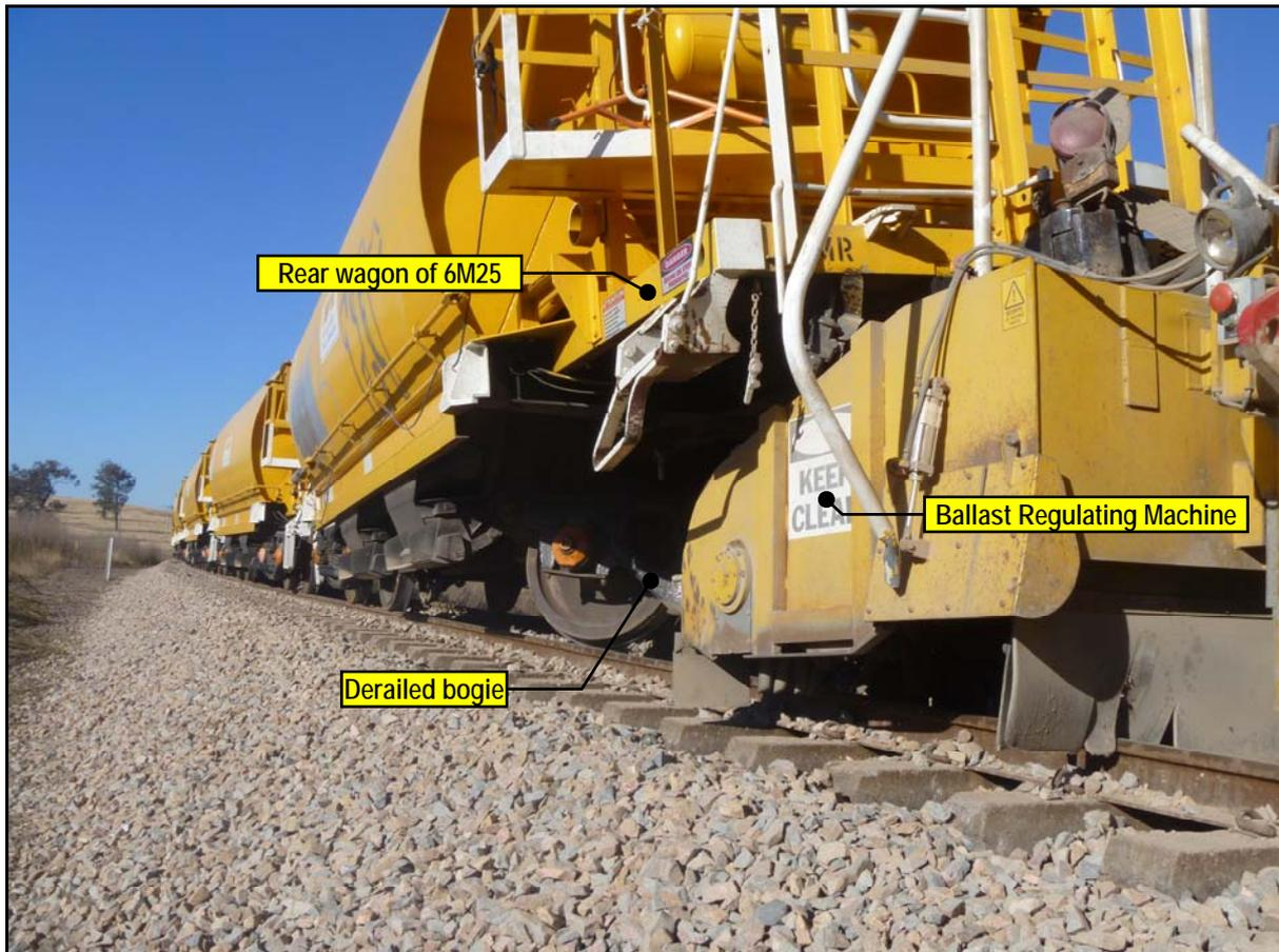
**Photograph 1: Position of rear wagon after colliding with the ballast regulating machine**
