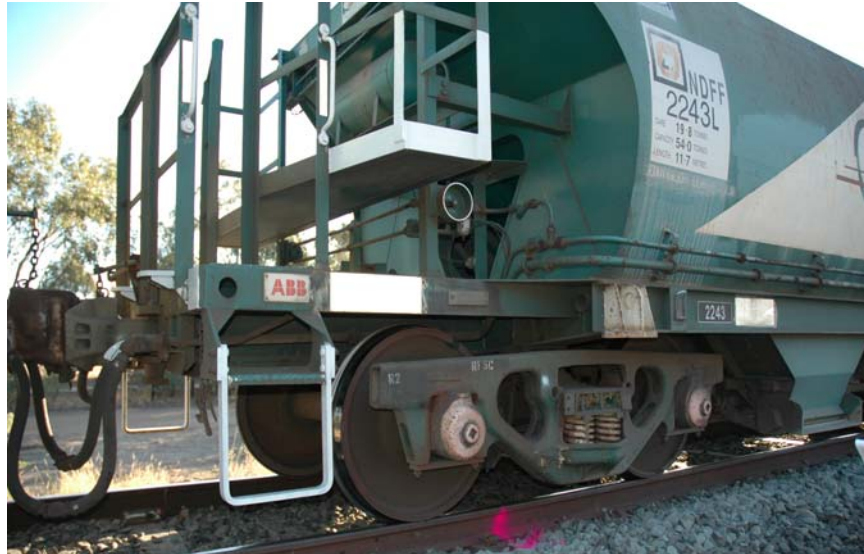
Figure 2: Ballast Wagon Walkway and Steps
