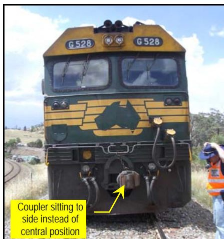
Photo 3: Position of front automatic coupler indicating the extent of lateral forces.
