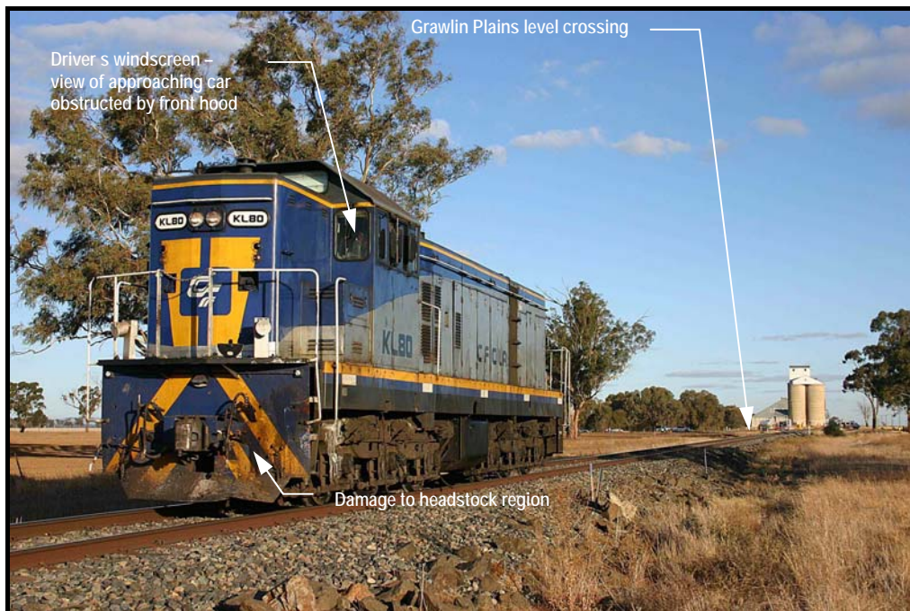
Photo 3: Locomotive's position after the collision
