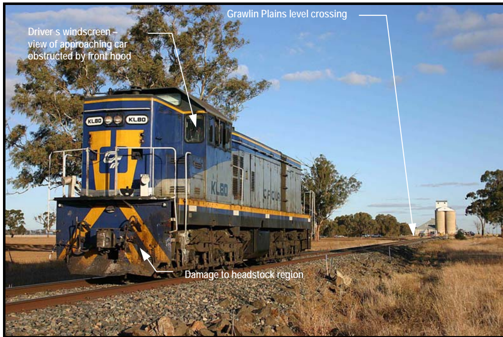
Photo 3: Locomotive's position after the collision
