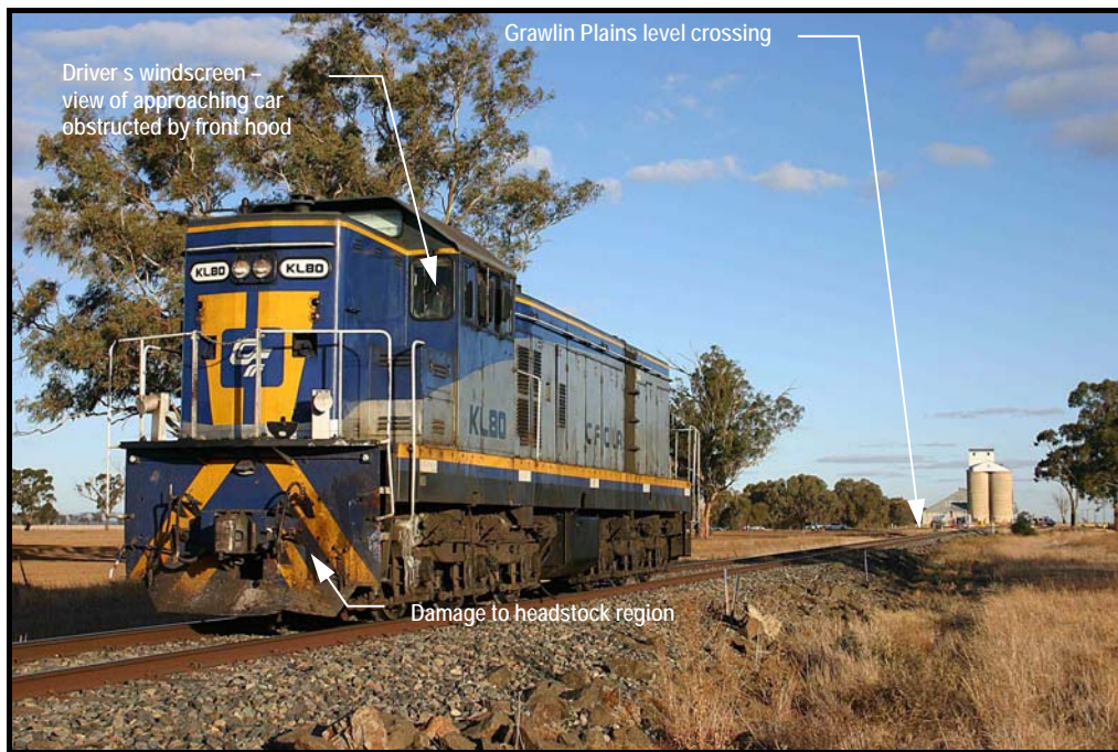
Photo 3: Locomotive's position after the collision
