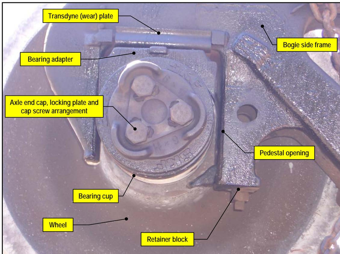
Photo 3 Typical Wheel and Bearing Components
