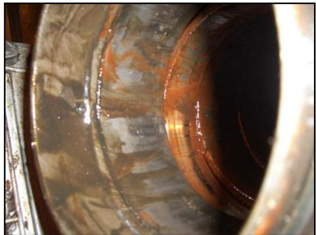
Photo 11 Condition of Lubrication in the 'Mate' PUB on 1WB3 (Wauchope)
