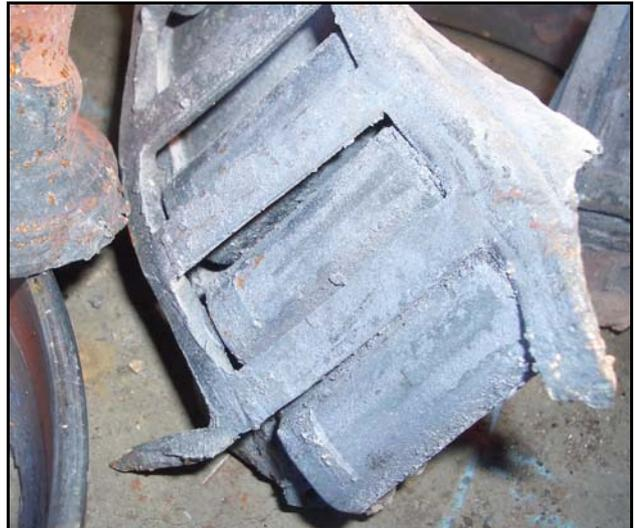
Photo 9 Damage to Bearing Cone and Rollers from PUB off 1WB3 (Wauchope)
