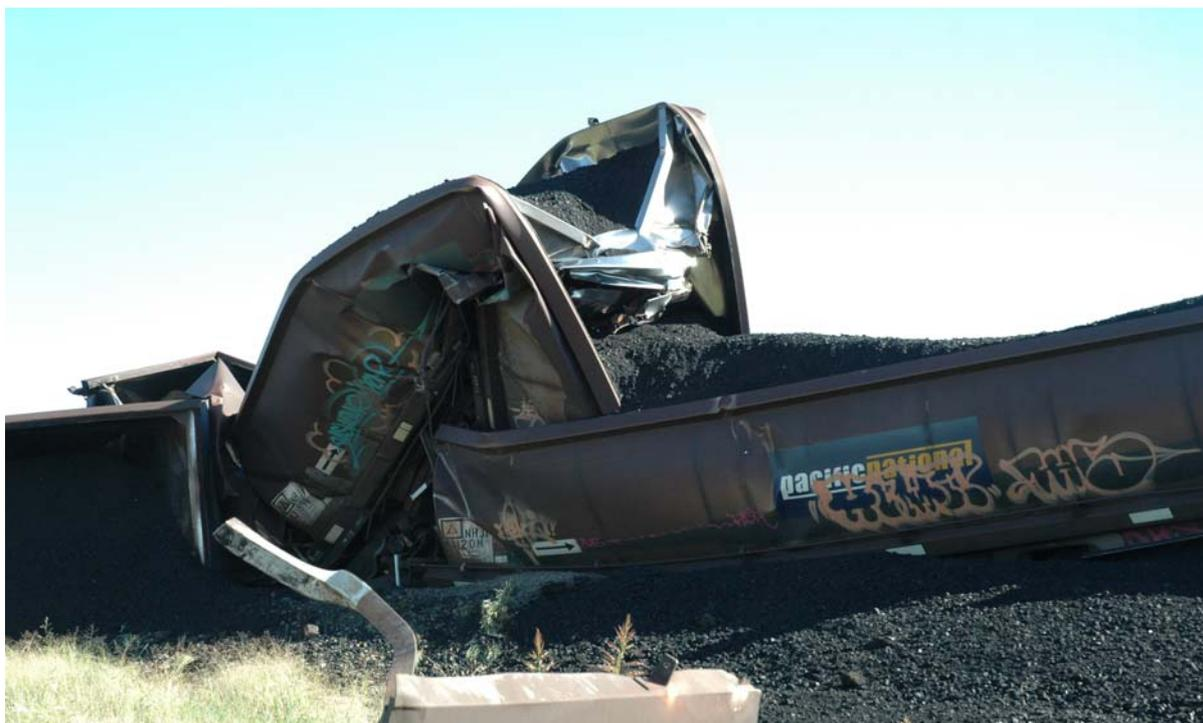
**Photograph 2: Indicative damage to derailed wagons**
