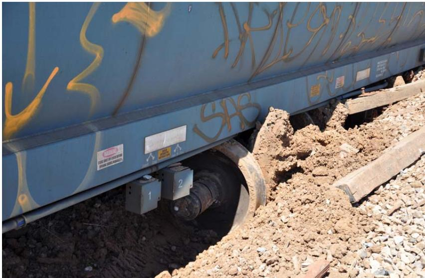
**Photograph 3: Wheel from the 36<sup>th</sup> wagon acting as a plough**
