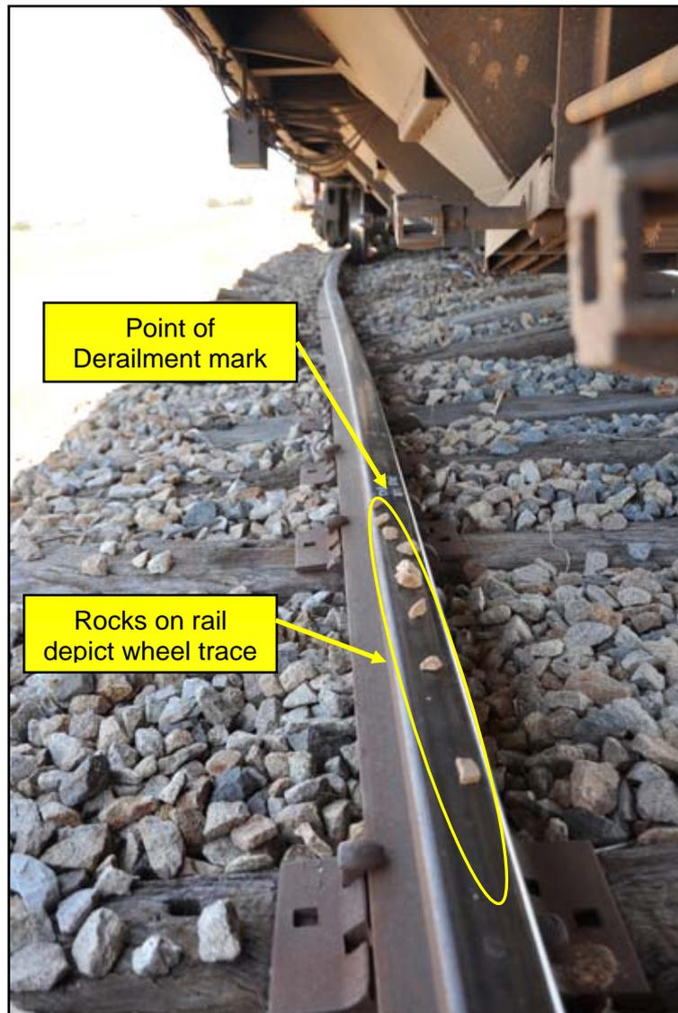
**Photograph 1: Point of derailment marks on the Up rail**
