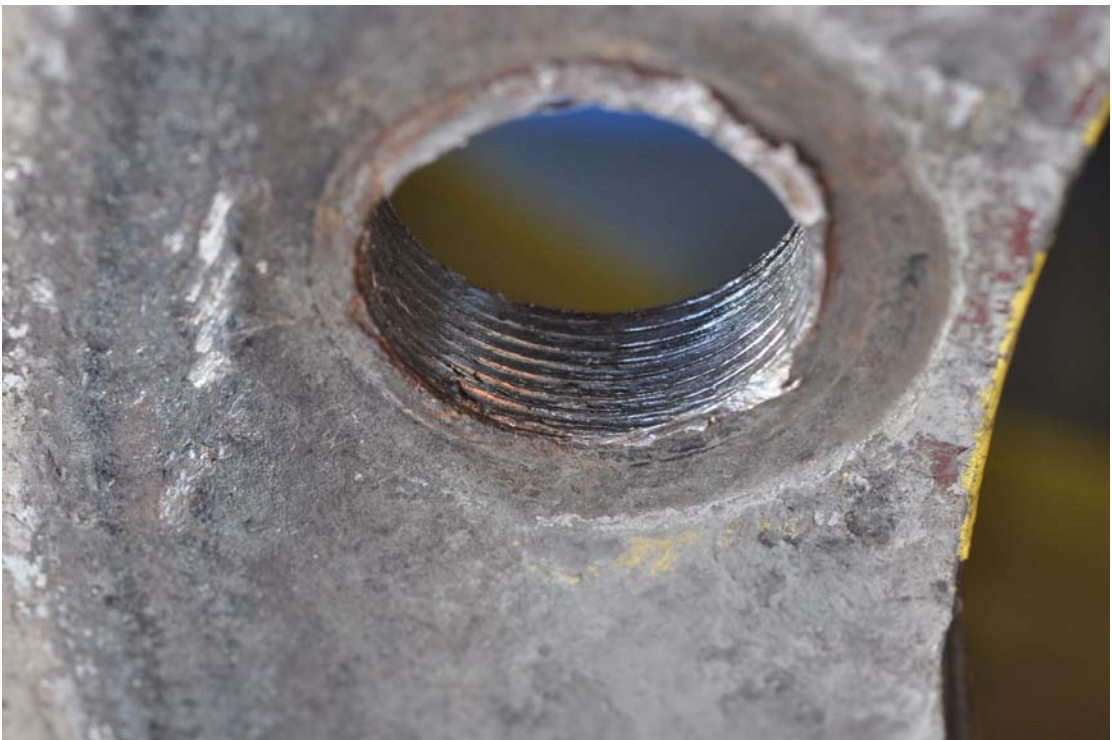
Photograph 2: Damaged Inner Rim Stud Hole
