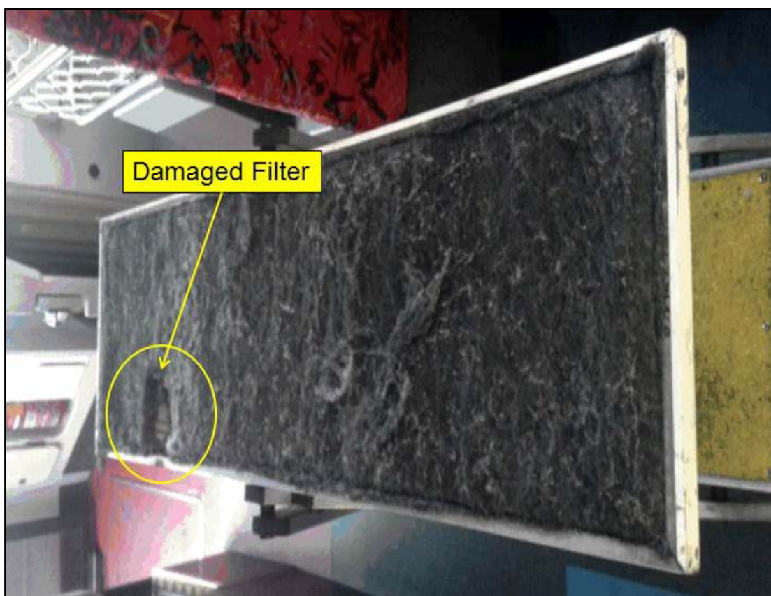
Figure 1: Fire damage to air conditioning filter
