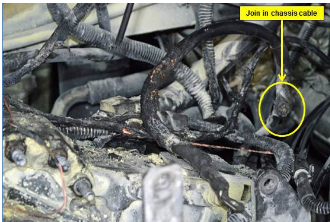
Figure 5: Alternator cable, showing the join where an extension was attached
