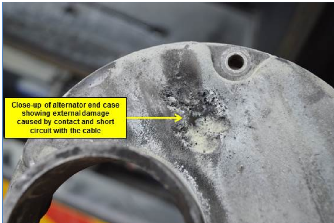
Figure 7: Exterior of the alloy alternator end case.
