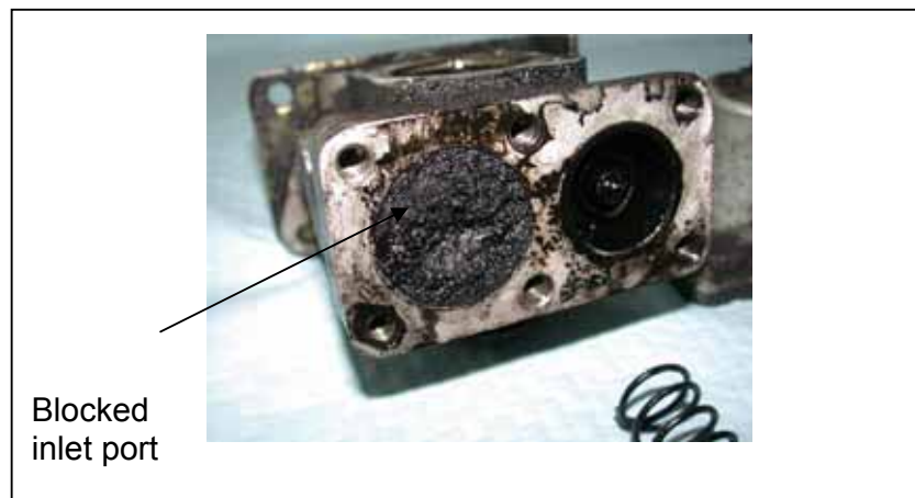
Figure 4: Photograph of Unloader Valve Removed From MO8053 on 17/03/2004
