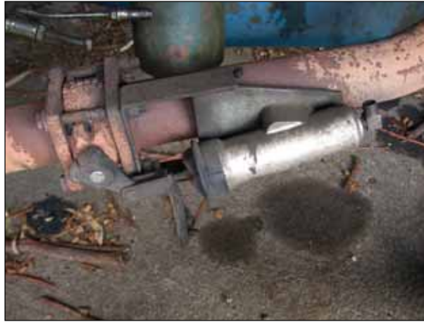
Figure 5: Photograph of Disconnected Exhaust Brake from MO8053 on 17/03/2004
