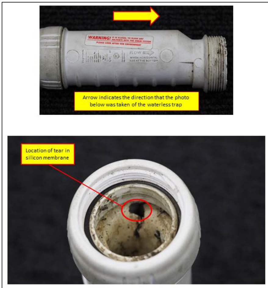
Figure 17: Tear in waterless trap sealing membrane
