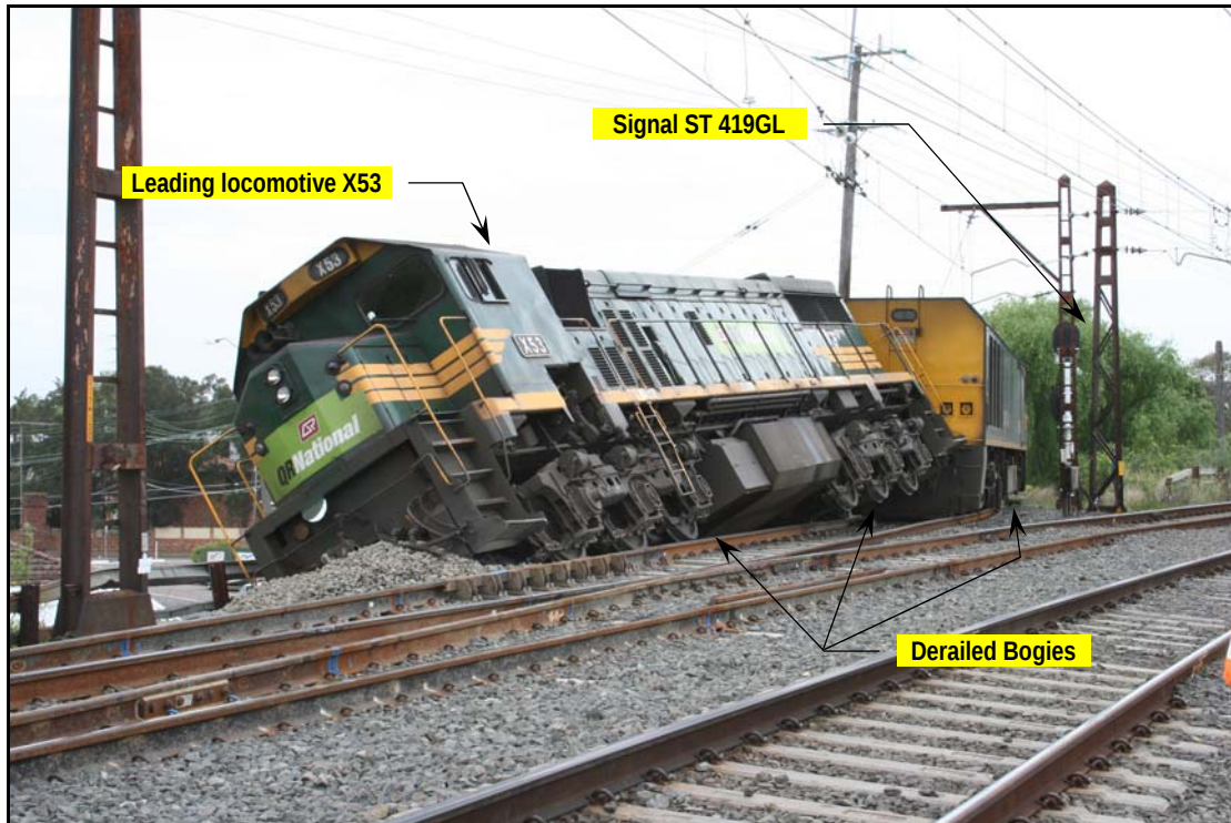
Photo 2 Derailed locomotives of 4BM7 at daylight on day of incident
