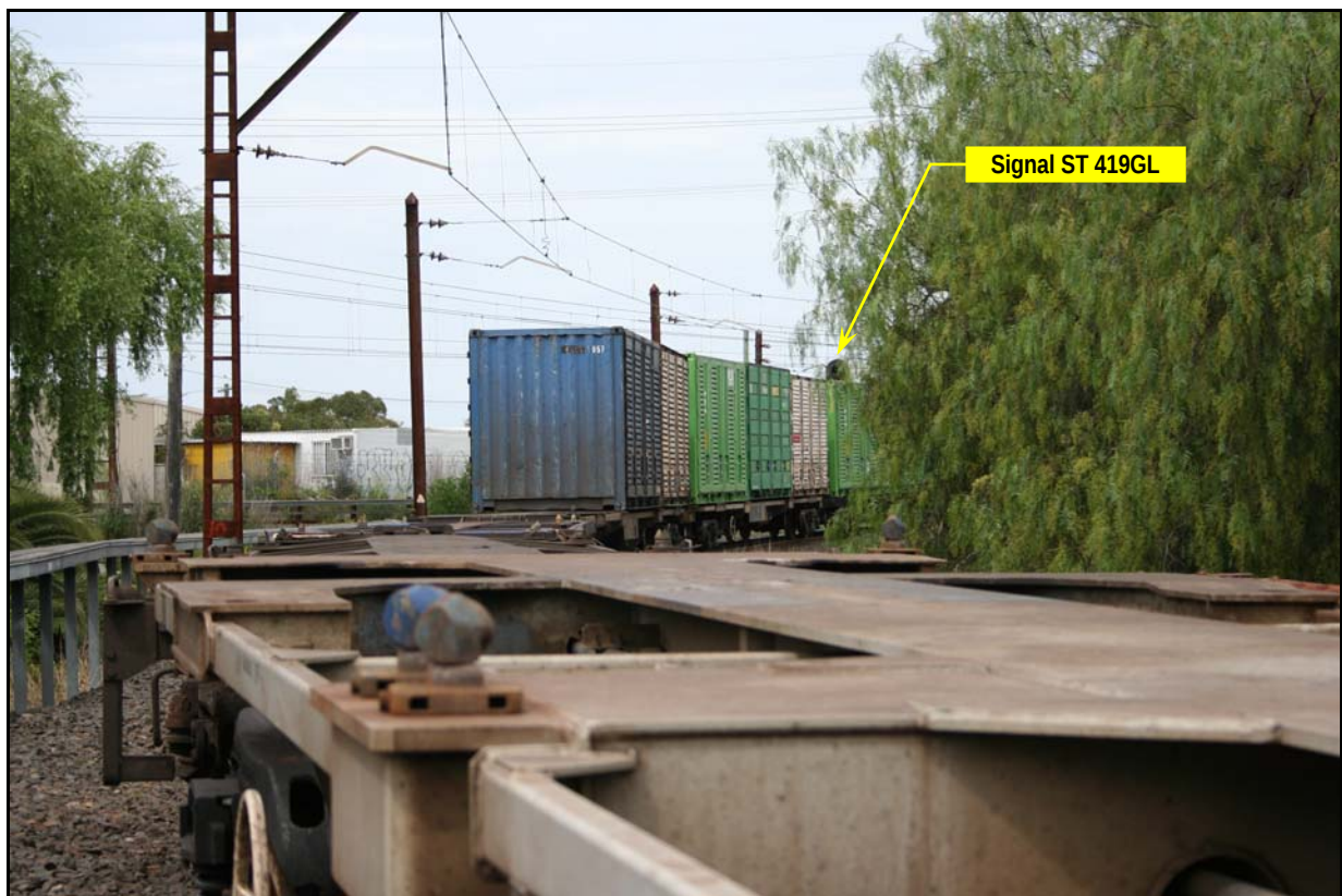
Photo 6 Point 93m from Signal ST 419GL, at which sighting first becomes unobstructed
