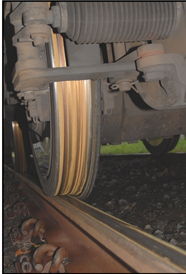
Photo 8: Evidence of rust emulsion and skid marks on the wheel and rail.
