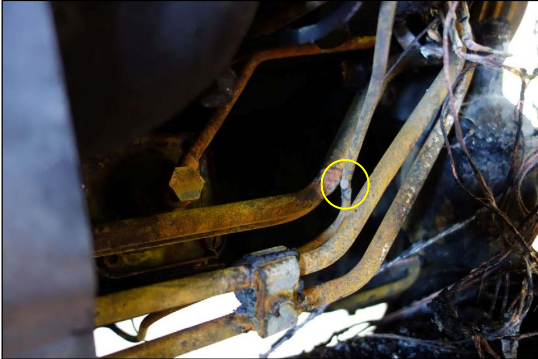
Photograph 4: Fuel return line in situ, showing previous repair
