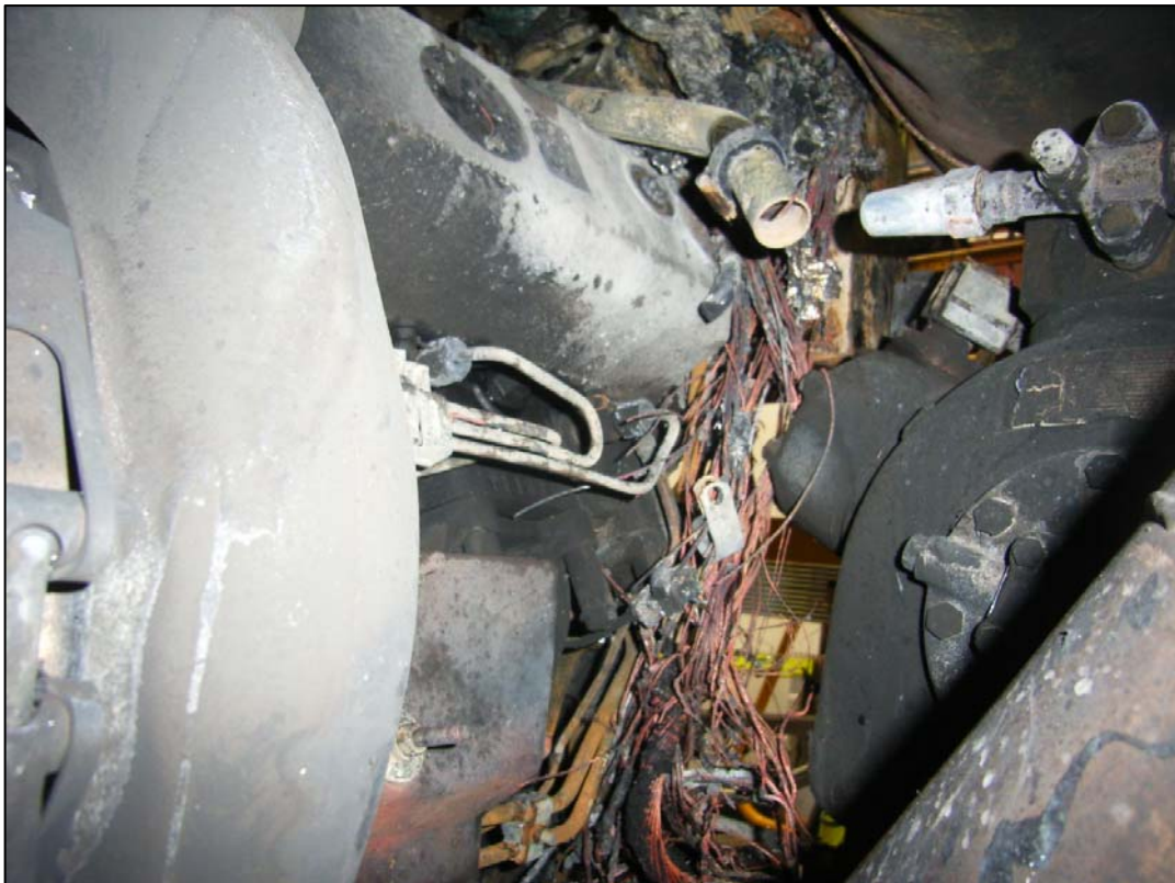
Photograph 3: Component damage adjacent to fuel return line
