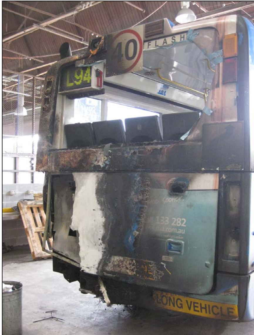
Photograph 1: Overview of fire damage to the rear of the bus
