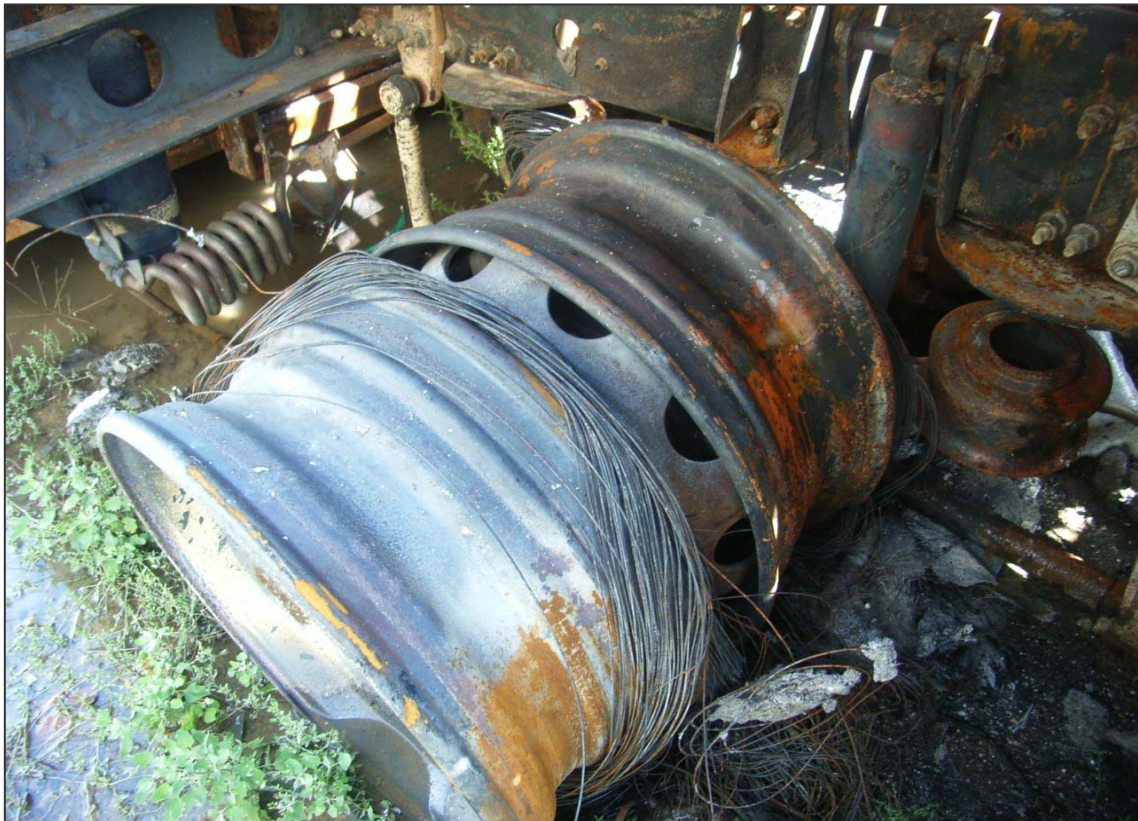
Photograph 3: Rear wheel rims showing location of steel tyre cord
