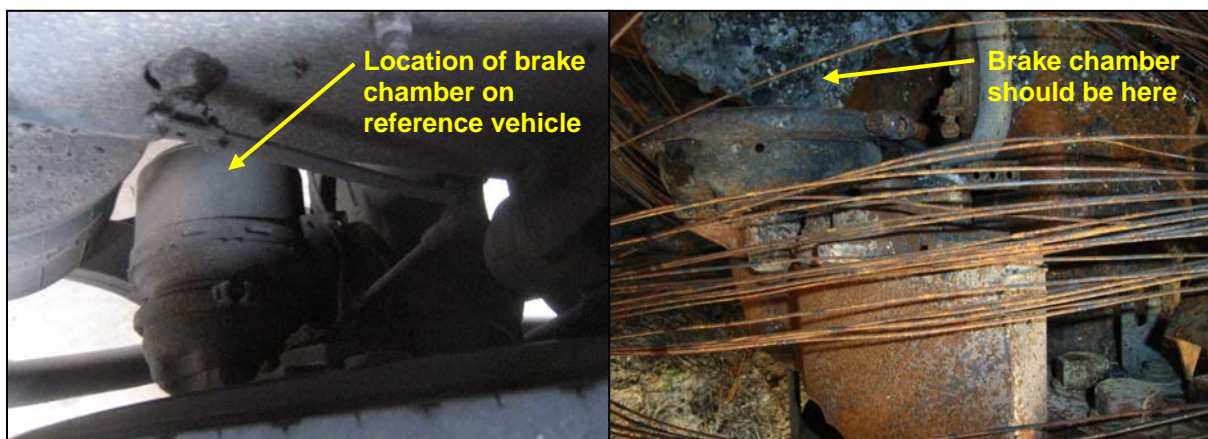
Photograph 5: Missing spring brake chamber
