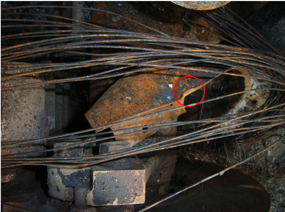
Photograph 7: Evidence of impact damage on edge of deformed brake shield
