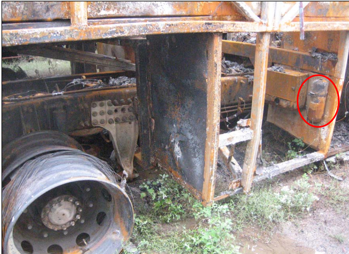
Photograph 8: Position of second (rear) fire extinguisher in relation to rear wheels
