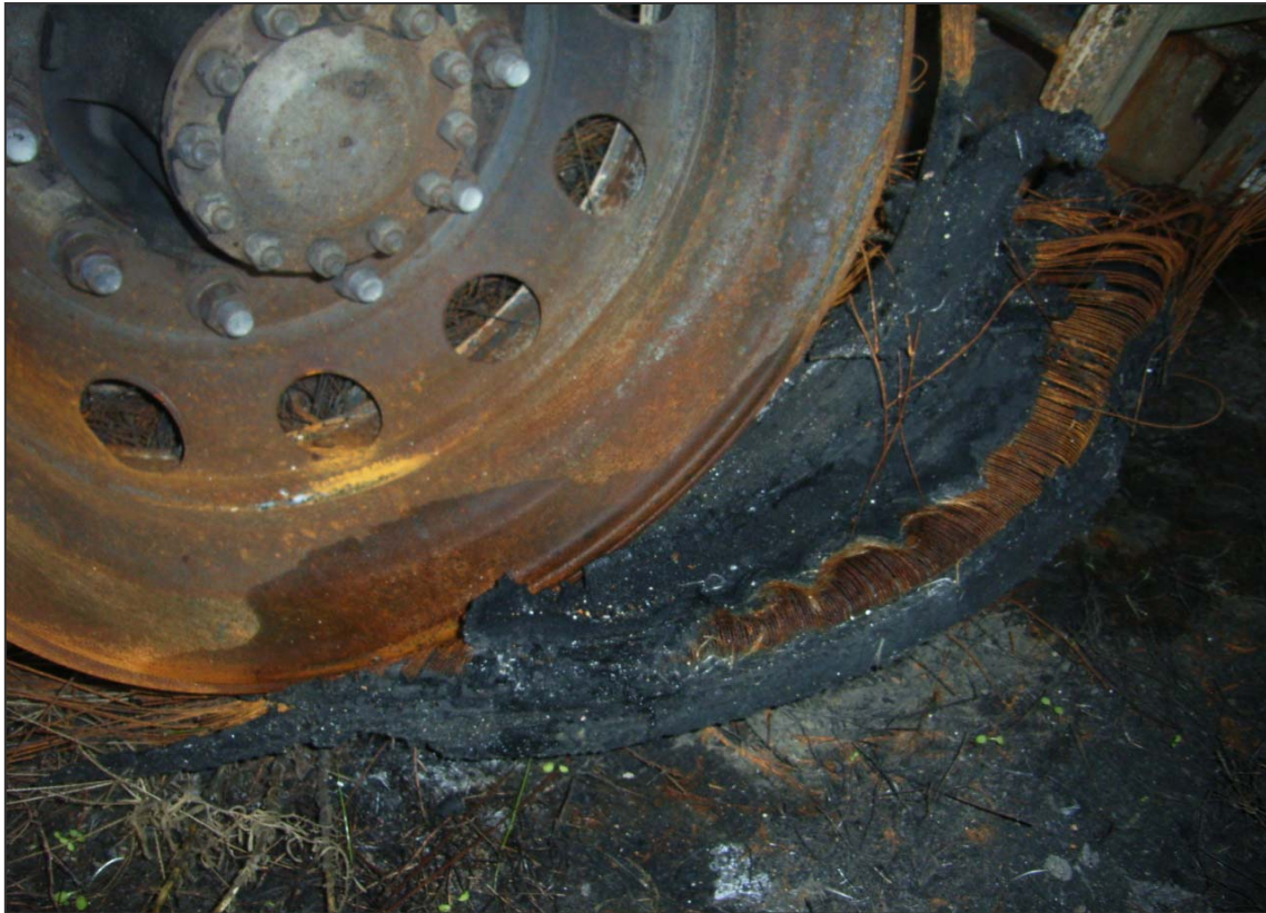
Photograph 4: Remaining rubber from right outer rear tyre
