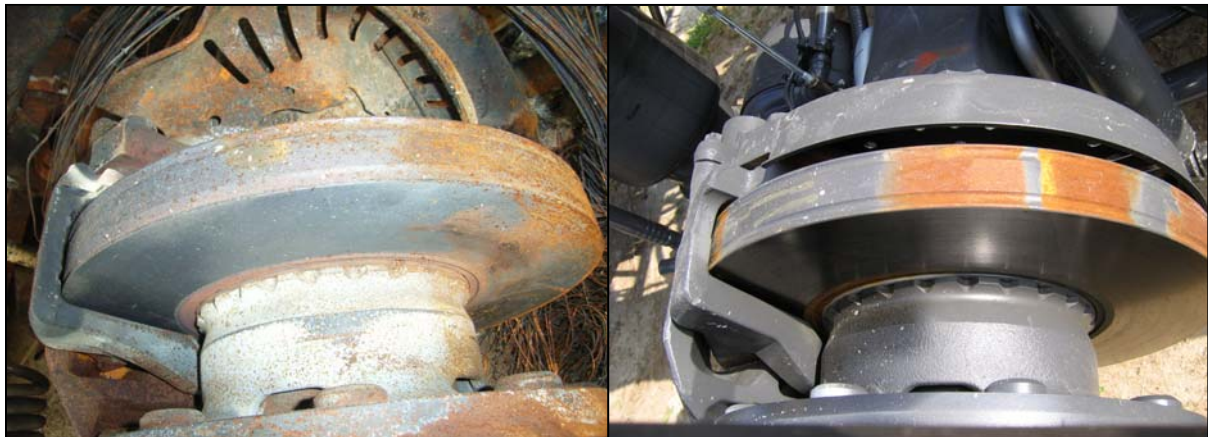
Photograph 6: Comparison of the damaged shield (left) with an undamaged shield (right)
