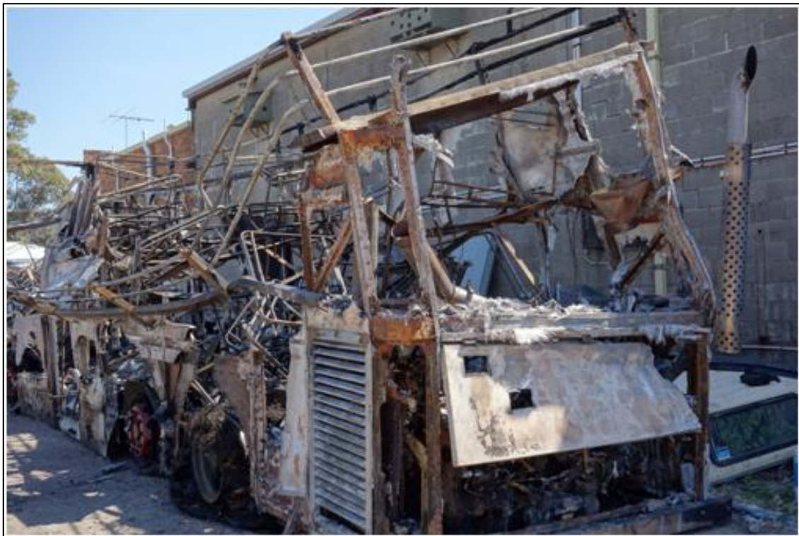
Photograph 2: Post-fire condition of bus
