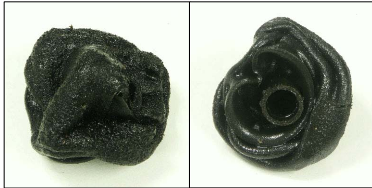
Photograph 17: Heat distorted oil filter venturi
