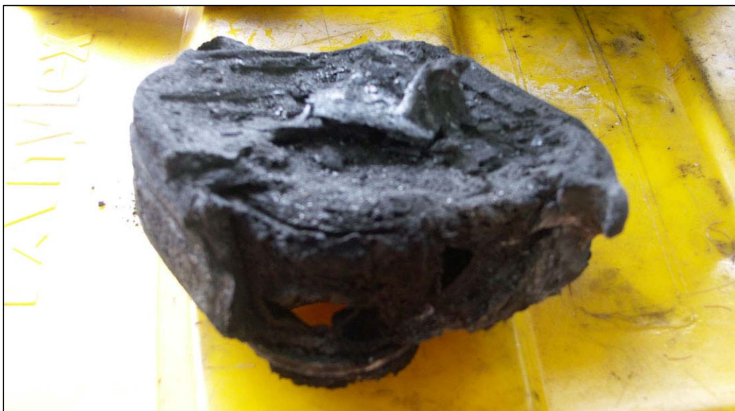
Photograph 6: Damaged engine control module after removal
