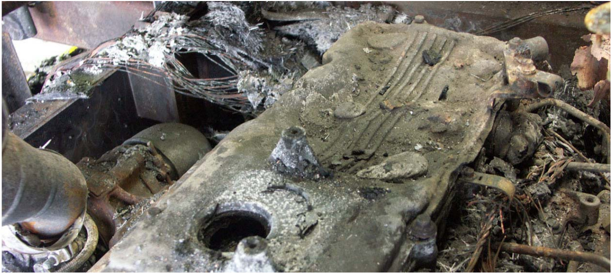
Photograph 19: Heat damage to the cam cover
