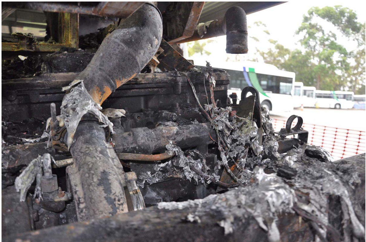
Photograph 18: Damage near turbocharger
