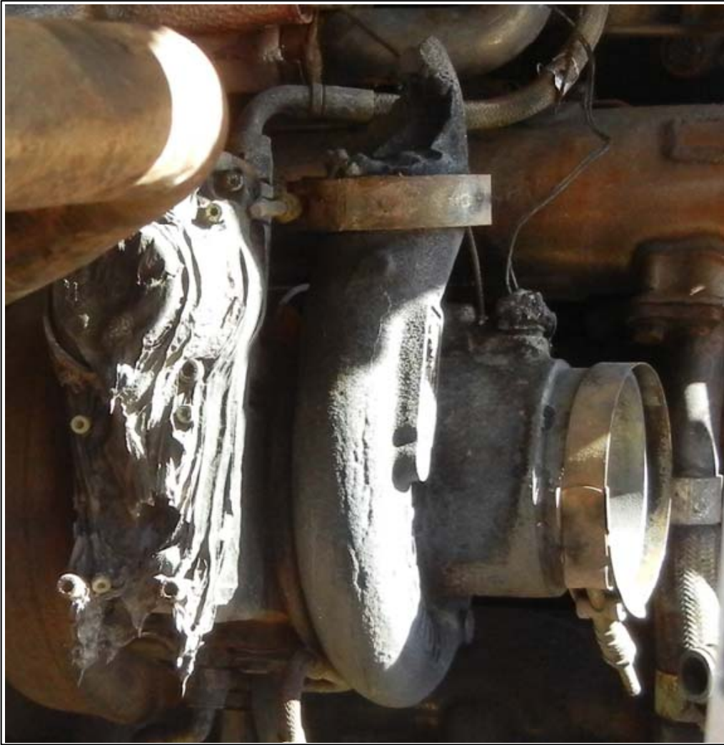
Photograph 6: Heat damaged alloy turbocharger
