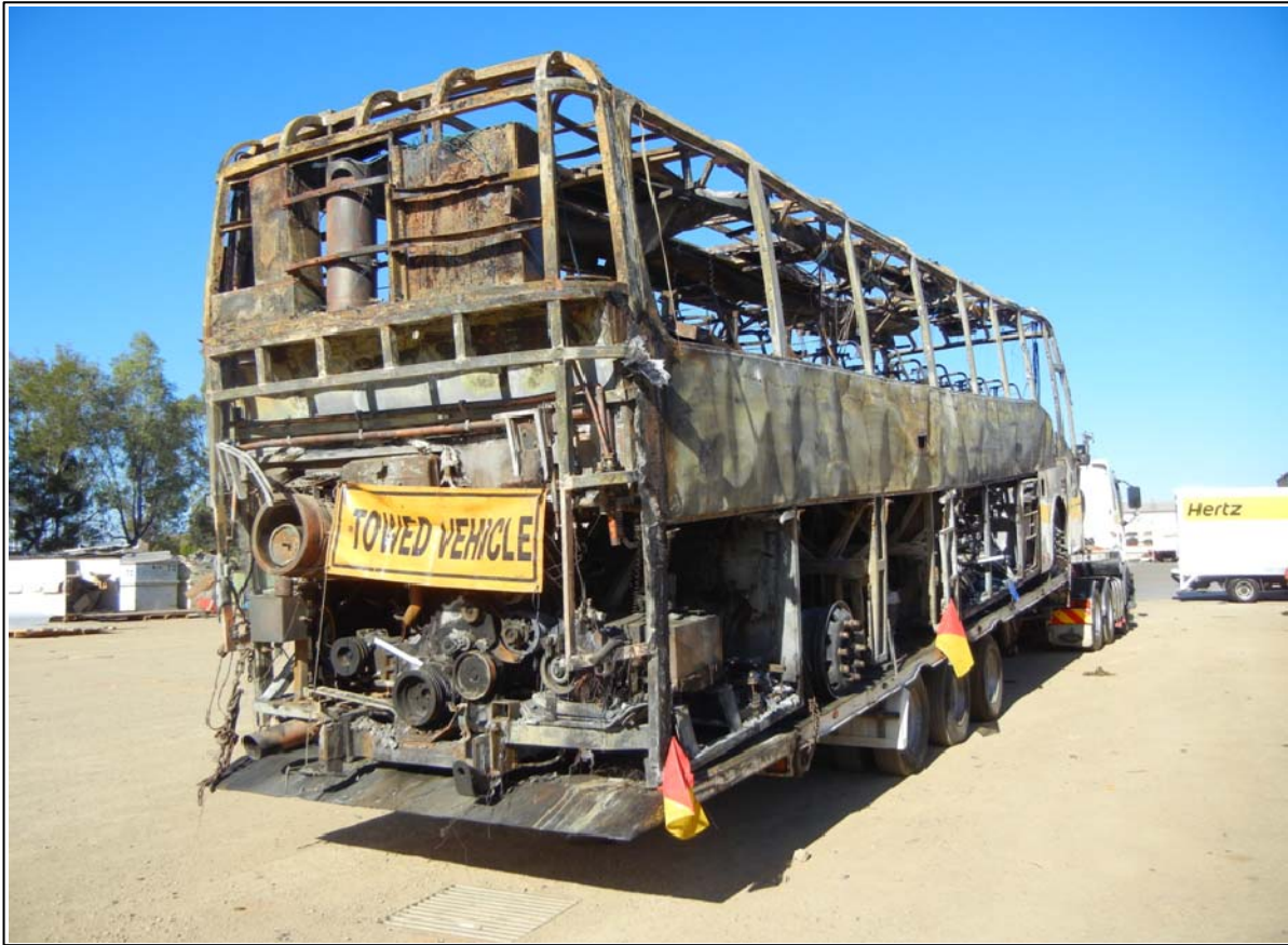
Photograph 2: Post-fire condition of bus
