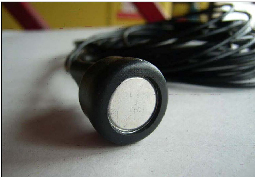
Photograph 9: Fire warning sensor fitted to B7R coaches
