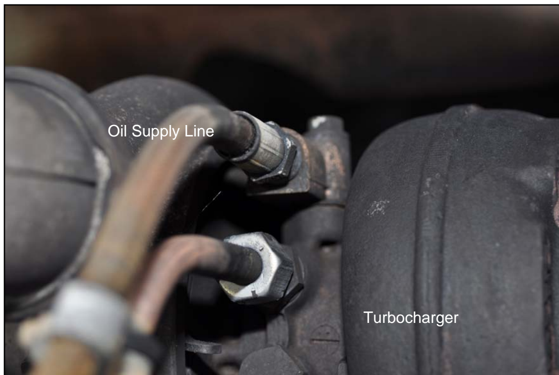
Photograph 3: Main oil supply oil line sitting within flange unit but not secured
