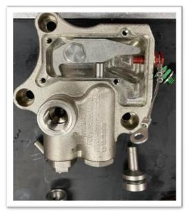
Left image: Picture of disassembled valve body showing the internal function of the red isolation screw.
