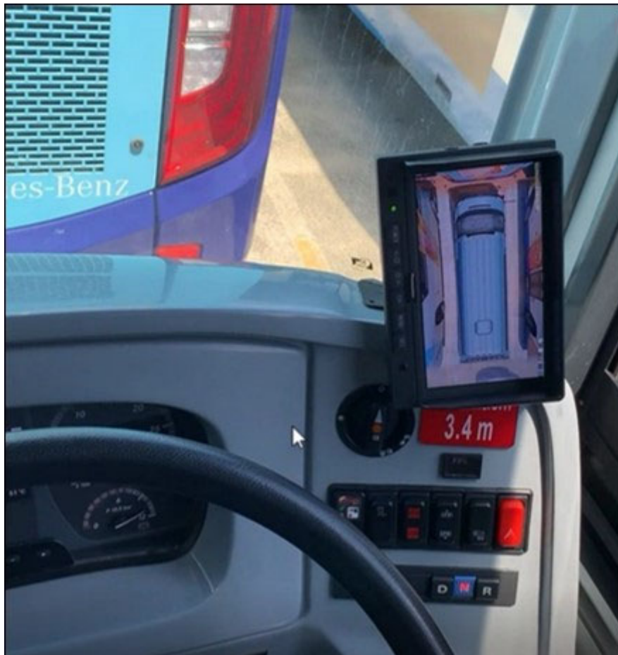
Figure 13: Transit Systems trial 360° external camera system
