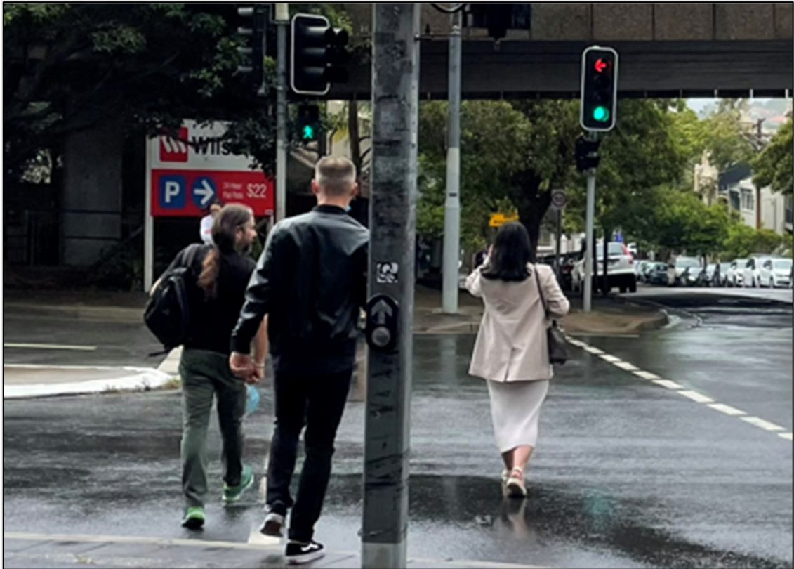
Figure 14: Grosvenor/Grafton Street Pedestrian Crossing with red arrow pedestrian protection on activation of green walk signal fitted post incident
