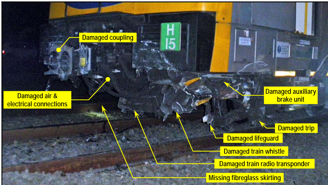
Photograph 6: Equipment damaged on leading car (6931) by the RMV
