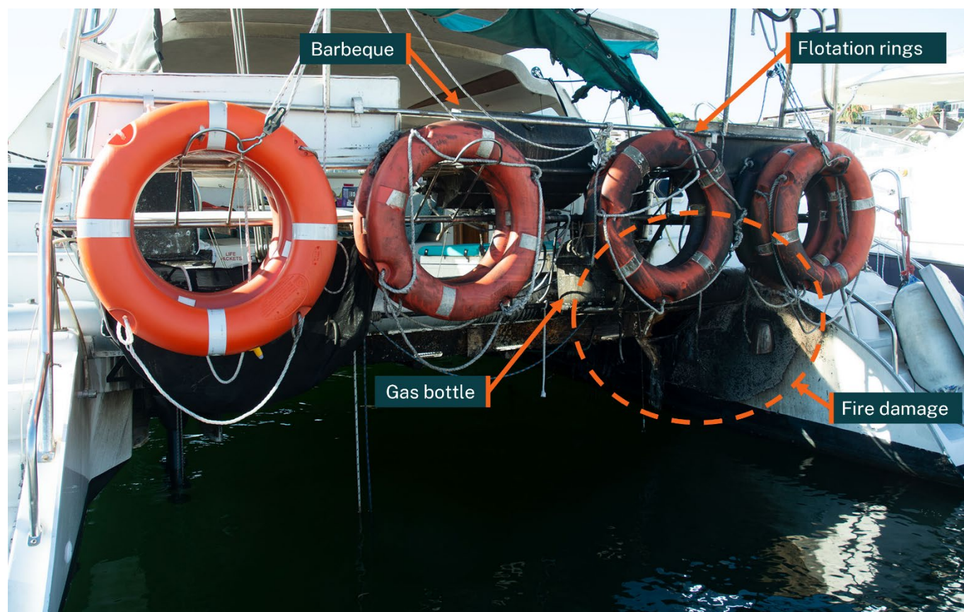
Figure 1: Flotation rings and fire damage
