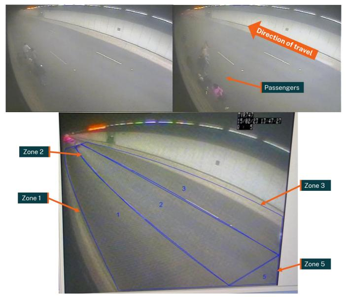
The upper images shows the pedestrians that were not initially detected as seen from camera TVR747 with the lower image showing the pedestrian detection zone for the camera. Source: Transurban, modified and annotated by OTSI
