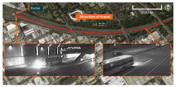
The image shows the path travelled by bus m/o9340 before entering the tunnel in Lane 1. The two inset images show the fire as viewed from the roadside cameras, initially as glowing on the road surface and then visible flames at the rear of the bus as it was entering the tunnel.
