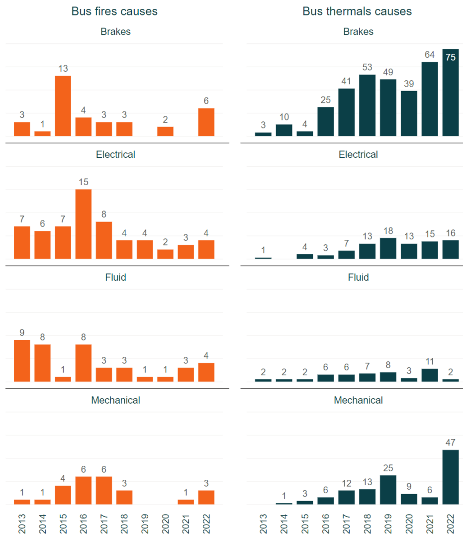
Figure 18: The year-by-year distribution of the different causes of the bus fire and thermal incidents in NSW over the last decade. Note that, ~9% of the fire and 2% of thermal incidents had “other”, “tyre” or “unknown” reasons and have not been shown in this figure.
