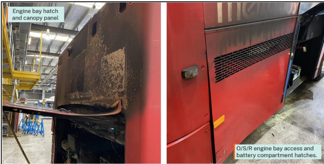
Figure 7: Damage to rear exterior of bus
