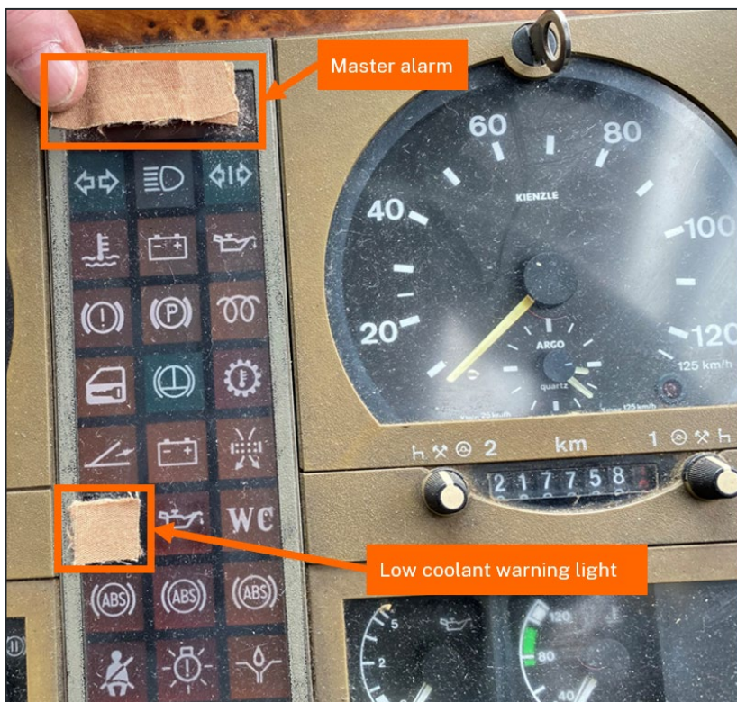
Figure 6: TV5251 dash alerting panel showing alarm lights covered at time of incident
