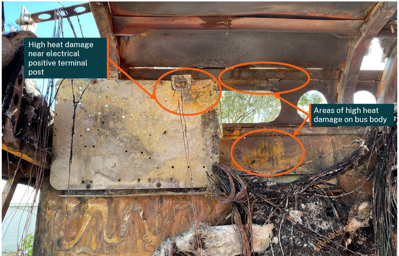
Figure 22: Heat damaged Accessory Panel
