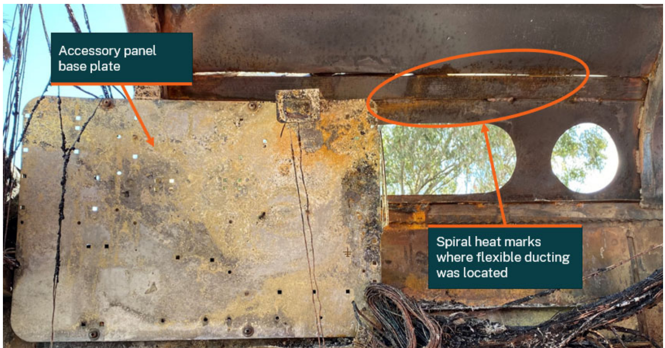
Figure 25: Spiral heat markings on bus body
