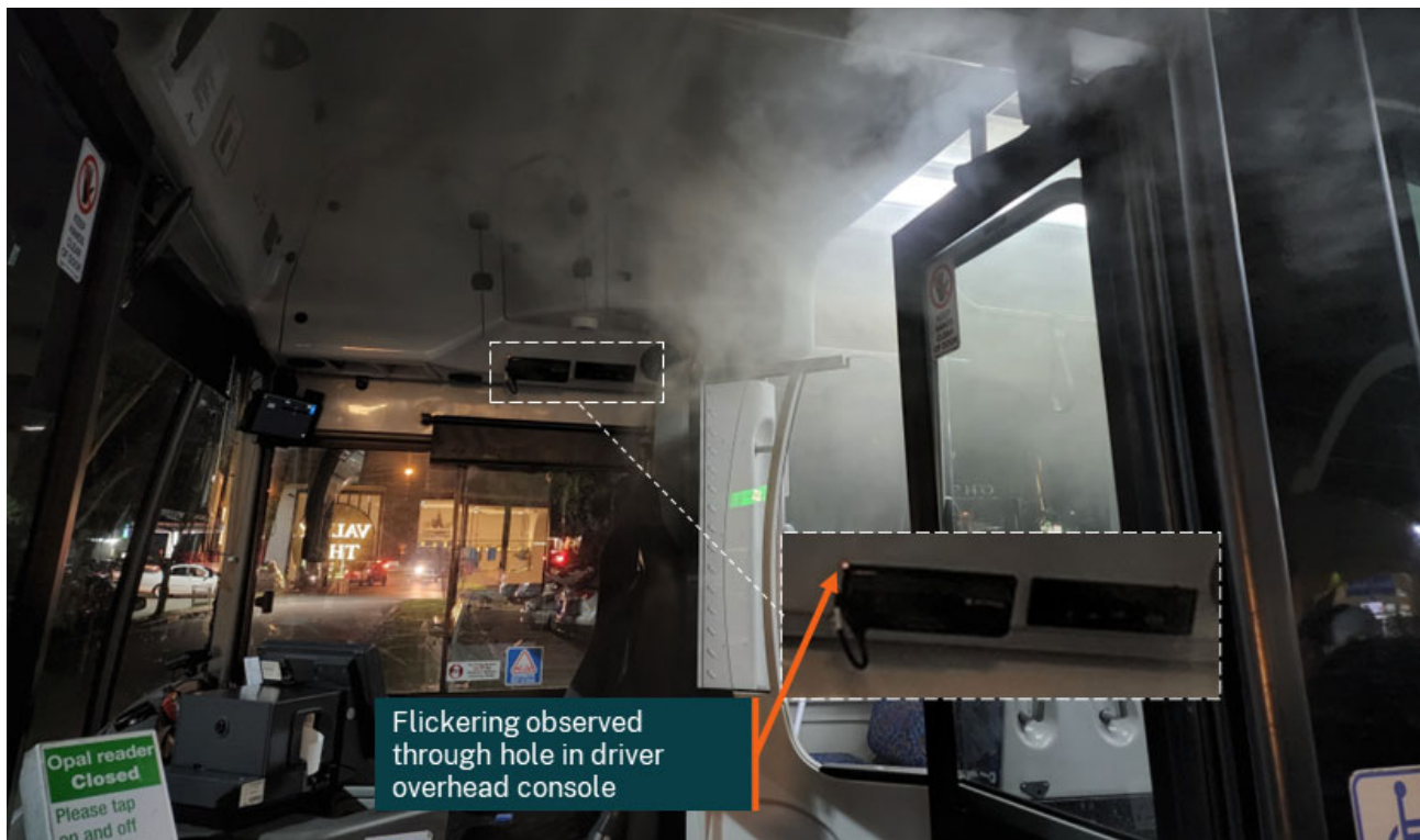
Figure 1: Illumination in the overhead console observed by the driver
