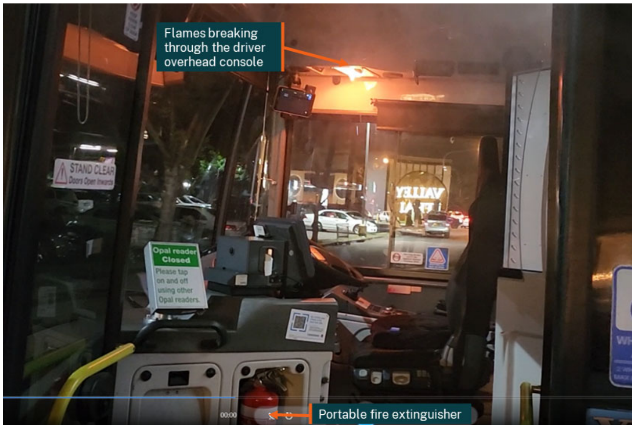
Figure 2: Flames breaking through the overhead console panel
