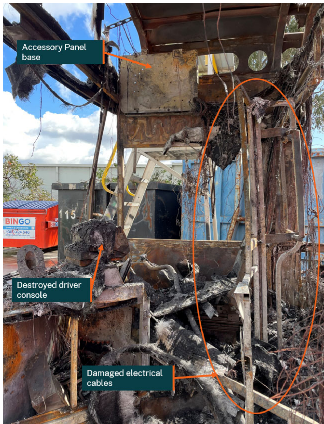
Figure 21: Damage to driver's position and overhead Accessory Panel
