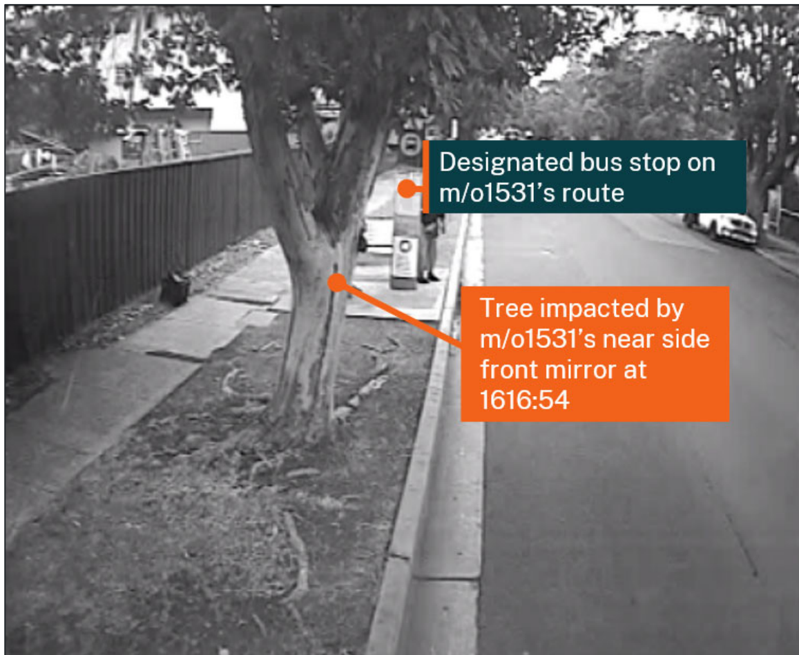
Figure 3: Recorded position of bus m/o1531 at 1616:54 from the forward-facing CCTV camera, immediately before mirror impact with the tree
