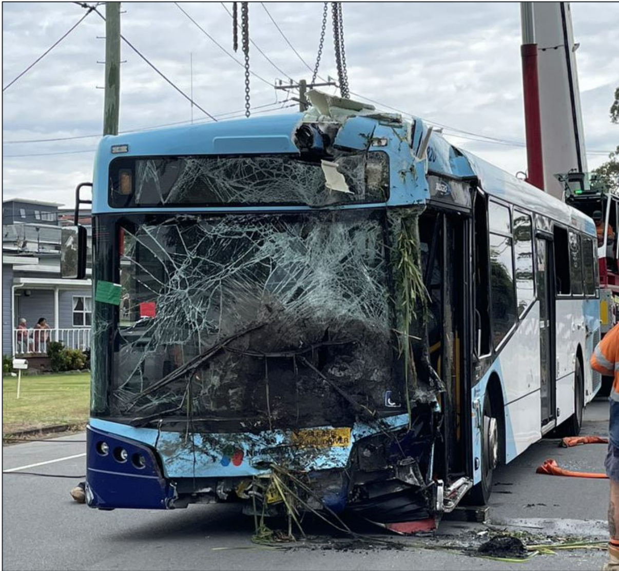
Figure 9: Image of bus m/o8219 during vehicle recovery process, showing impact marks and front damage
