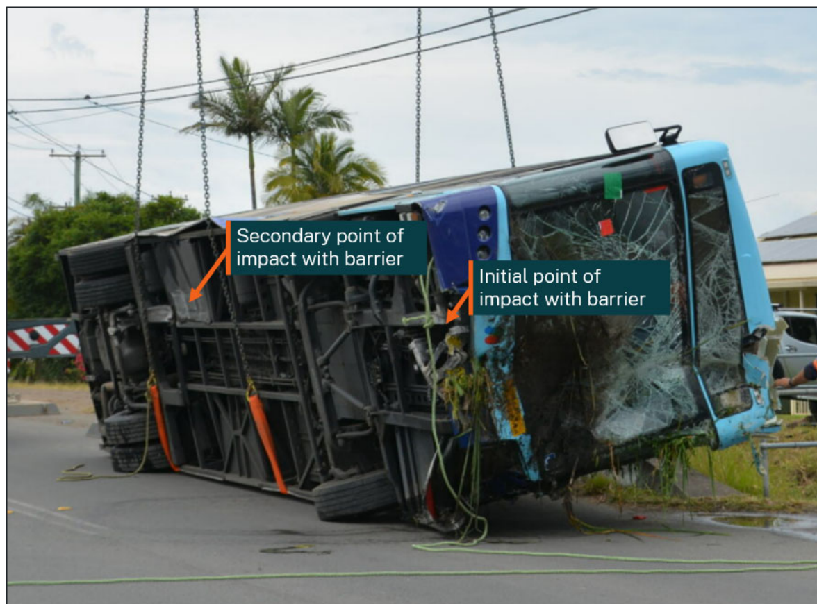
Figure 10: Image of bus m/o8219 in rollover position showing initial and secondary impact marks
