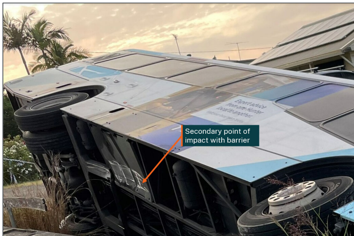
Figure 11: Image of bus m/o8219 in rollover position showing secondary impact marks
