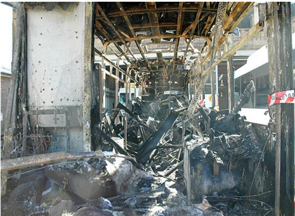
Figure 5: Fire damage to the bus interior.
