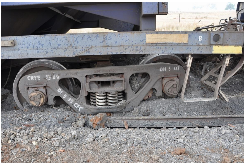
Figure 22: Poor quality ballast disturbed by the derailment.
