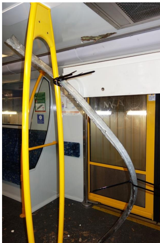
Figure 25: Angle iron secured inside the third carriage.
