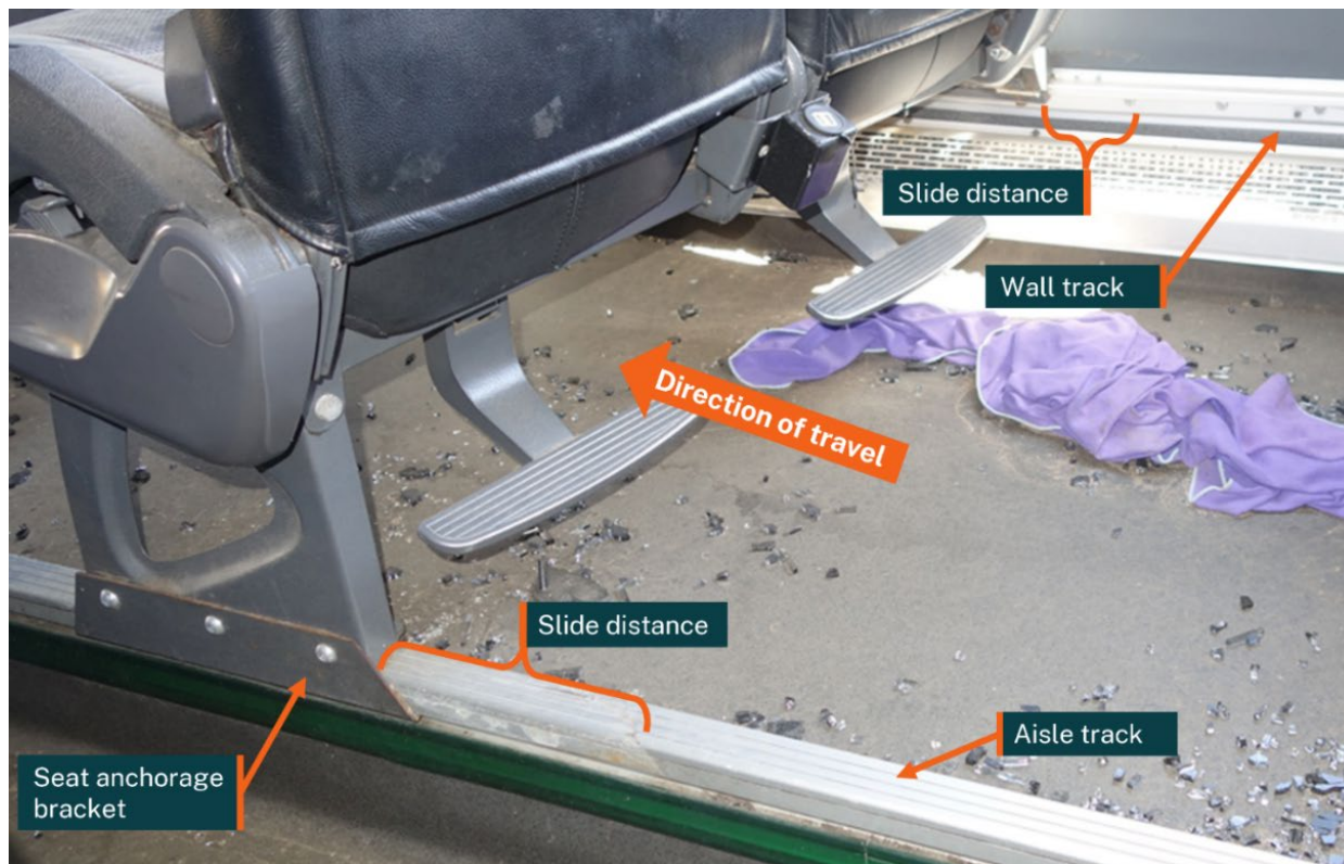
Figure 1: Seat slide and track mounting details
