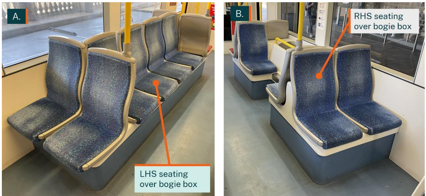
Figure 3: Urbos 3 C module carbody seating arrangements over bogie box
