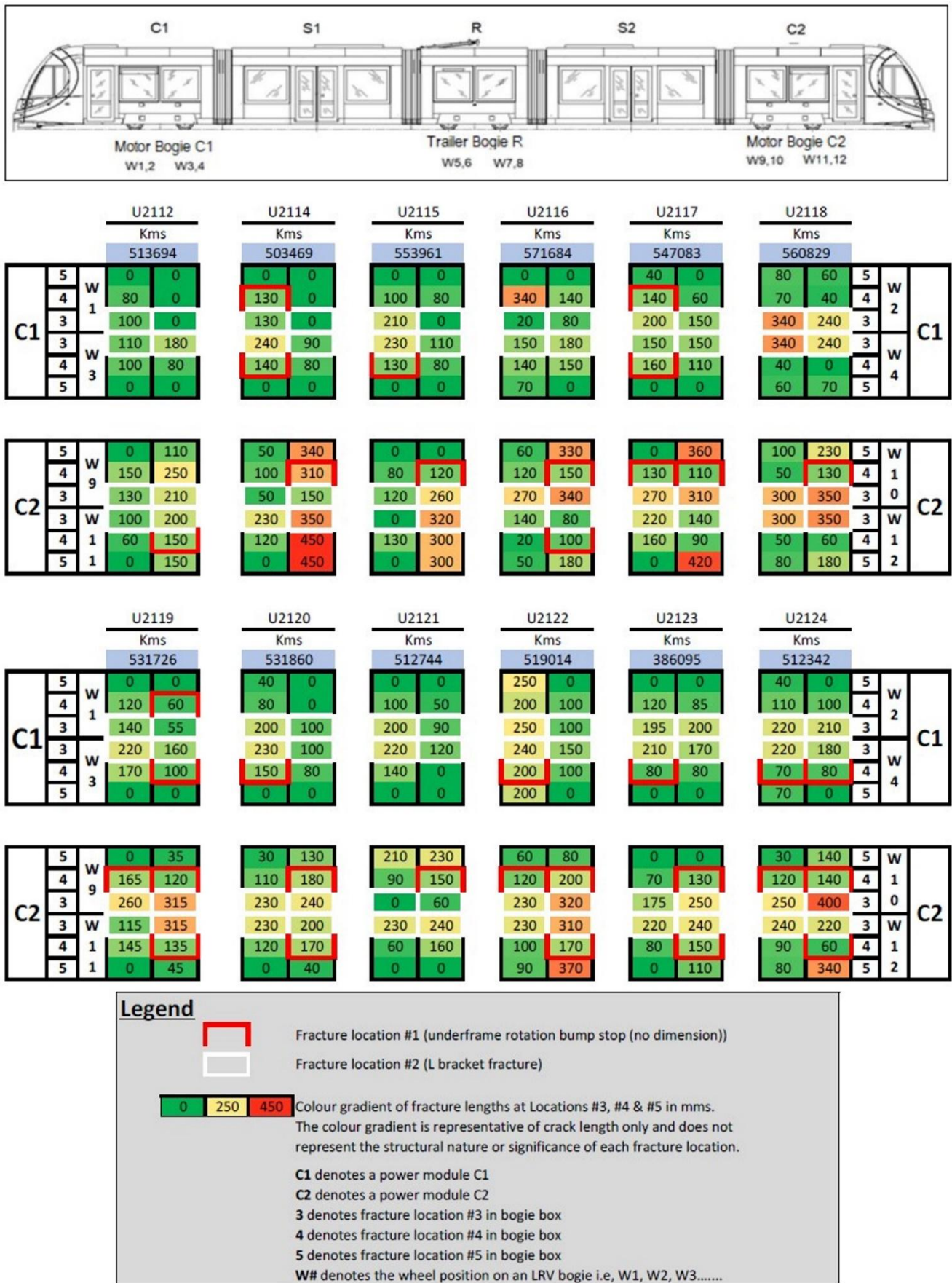
Figure 12: Urbos 3 unit fracture locations, measurements and LRV kms travelled
